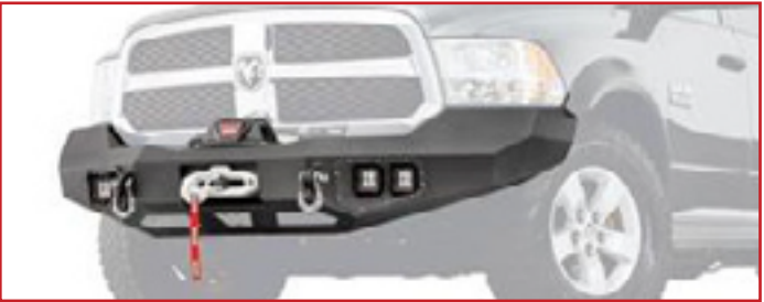
PRODUCT CODE: ULT100916 Bumper; Direct-Fit; Mounting Hardware Included; With Pre-Drilled Holes And Plugs To Accommodate Baja Grille Guard (Sold Separately); Without Grill Guard; With Winch Mount; With D-Ring Mounts; With Light Cutout; Textured Powder Coated Black Steel • OE bumper Sensor Compatible
