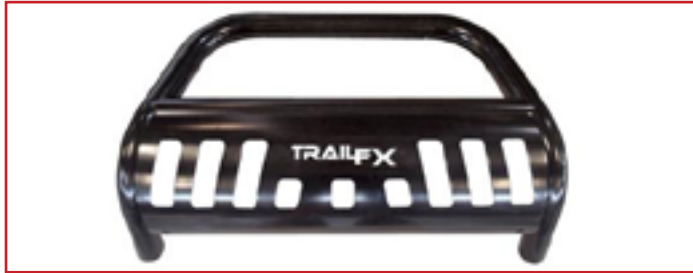
PRODUCT CODE: ULTB0028S Polished; Stainless Steel; 3 Inch Diameter; With Skid Plate; With Holes For Optional Lighting; 6.5 Inch Max Light/ 20 Inch Max Light Bar Tow Hooks Must Be Removed • Installation Will Interfere With Parking Sensors, Proximity Sensors, Forward Facing Laser Brake, Lane Keep Assist, Camera, and Cruise Control Sensors
