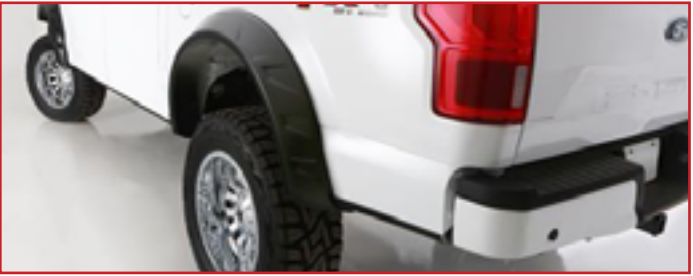
PRODUCT CODE: ULT20958-02 Fender Flare; DRT; Vented; 3 Inch Tire Coverage; Matte Black; Dura-Flex ® 2000 ABS; 4-1/2 Flare Height; Set of 4 • Position On Vehicle: Front and Rear • May Not Fit Vehicles With Technology Package (Sensors In Fenders)
