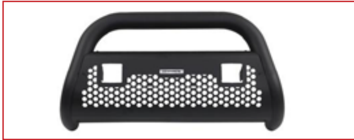
PRODUCT CODE: ULT55326T Charger- RC2 Light Ready; Black Textured Powder Coated Steel; 3 Inch Diameter; With 2 Bottom Light Mounting Openings; With Hexagonal Mesh Skid Plate; Requires Mounting Kit; Use Two 3 Inch Square Lights Installation Will Interfere With Parking Sensors, Proximity Sensors, Forward Facing Laser Brake, Camera, Lane Keep Assist, and Cruise Control Sensors
