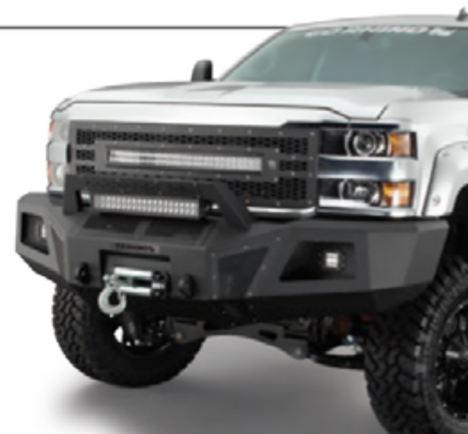
THUMB SCREW KIT GOR-24173T-1 Allows for Tool-Free Access to Winch Tray
