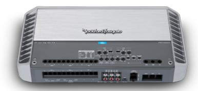
The PM1000X5 is a 1000 Watt 5-channel amplifier with high dynamic power using Class-a/b technology on the front/rear channels, Class-bd for the subwoofer channel, and a conformal coated pc board designed for motorsport and marine applications.
