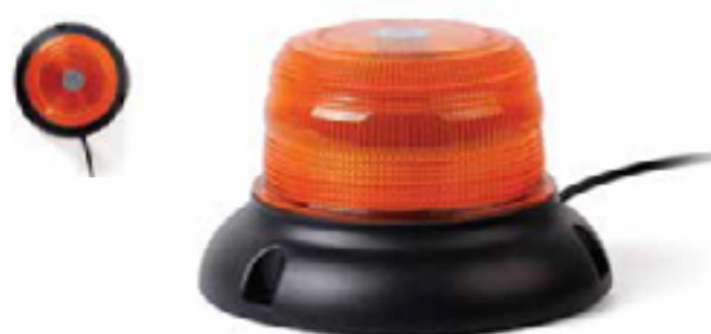
ULTXOA76512M LED Beacon - Magnetic Mount, Cigarette Lighter Socket, 7 Flash Patterns, Amber • Dimension: 5.12 x 3.19" • Source: 24x1.5W LED • Puissance / Power: 18W • Voltage: 9-30V • Protection: IP67 • Approval: ECE R65/R10 - SAE J845 - CAP 168
