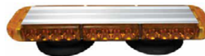
ULTE-2232AM 23" x 3 11/16" x 2 3/16" H • 12V - 30V. 12 flash patterns. 40 1W amber LEDs . Aluminum housing with polycarbonate amber lens. 2 magnets with suction cups. Cigarette power adaptor with switch for flash pattern selection & 12.5 ft of wire.
