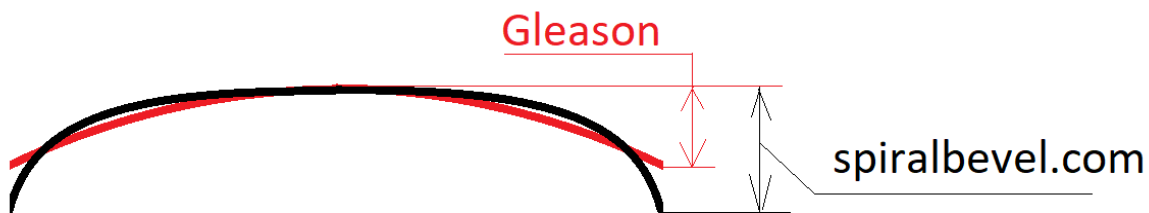
Picture 5. Spiralbevel.com contact localization method allows more room for errors in shaft misalignment.
