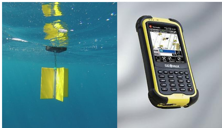
Figure 6. Drogue deployed at sea for current measurement (left) and hand-held GPS used to geo-reference sampling locations
