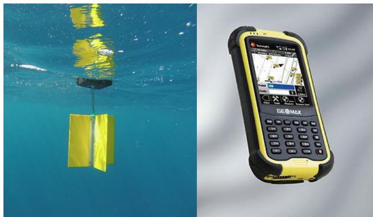
Figure 8. Drogue deployed at sea for current measurement (left) and hand-held GPS used to geo-reference sampling locations
