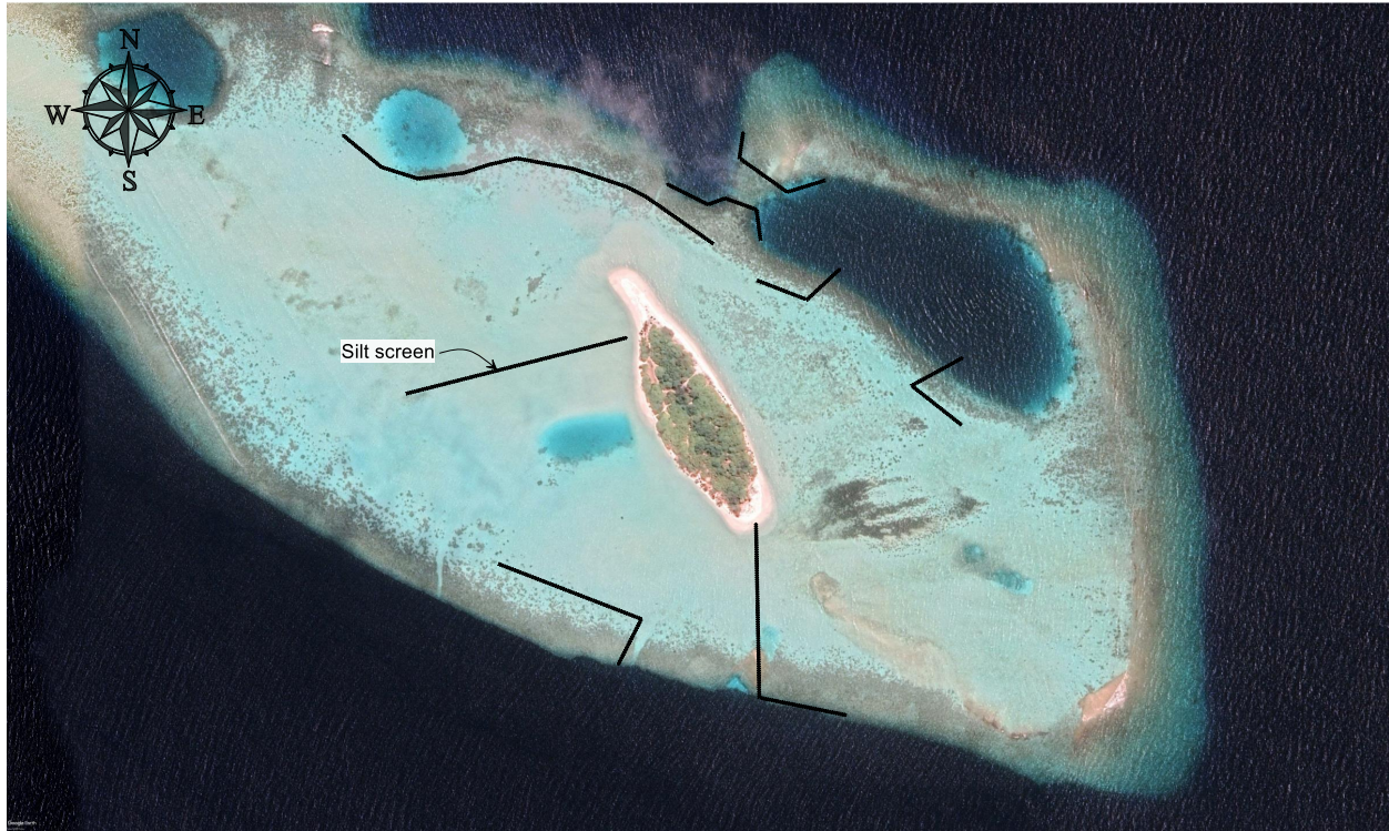
Figure 62: Potential location for placement of silt screens during construction of the resort
