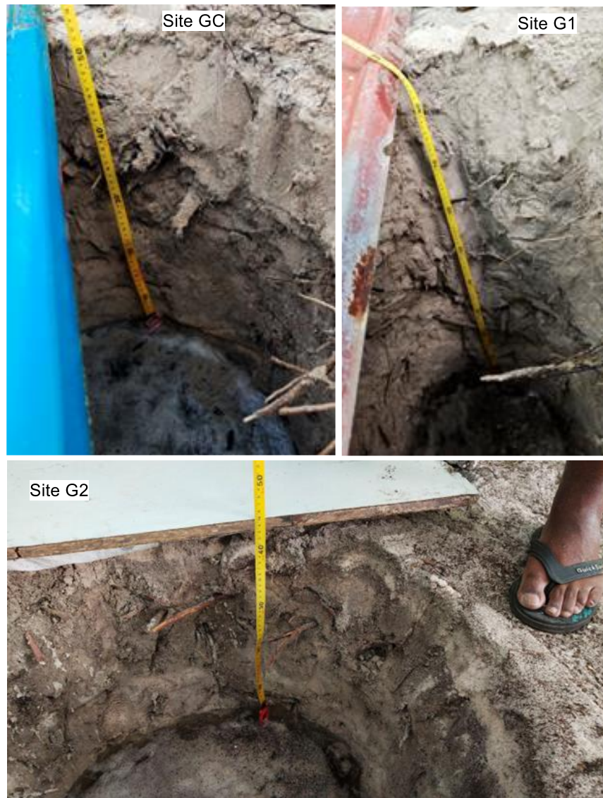
Figure 38: soil profiles at project site
