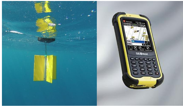
Figure 1: Drogue deployed at sea for current measurement (left) and hand-held GPS used to geo-reference sampling locations
