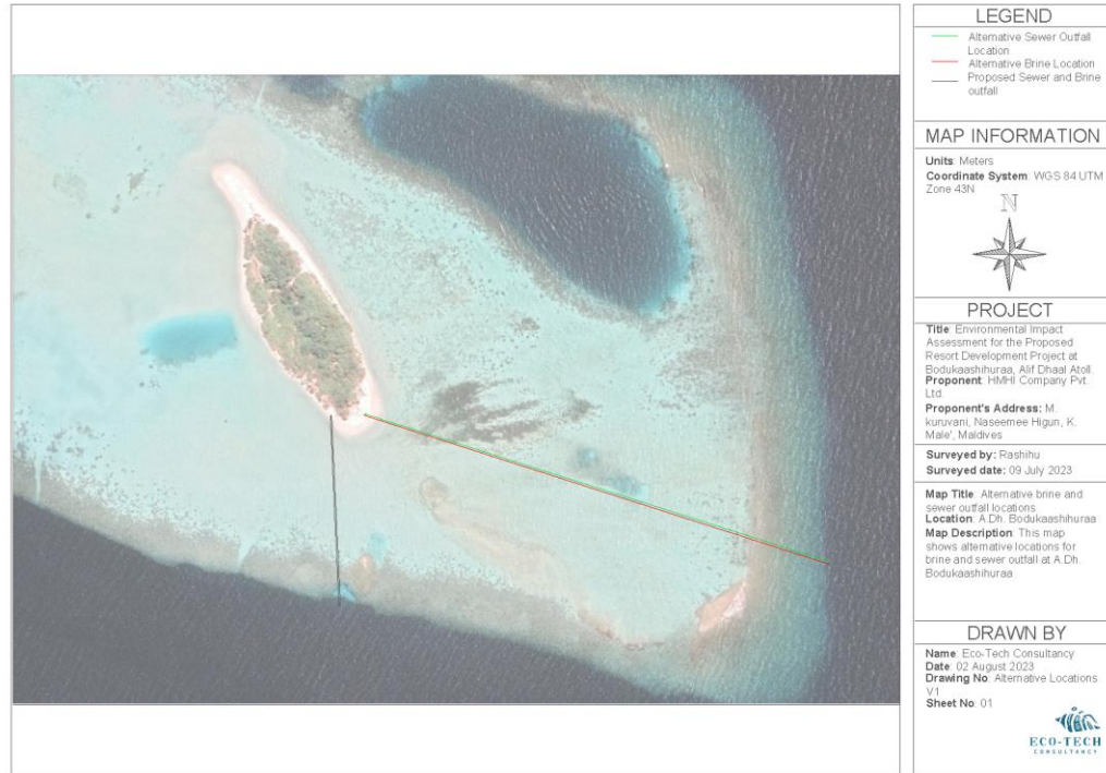
Figure 61: Alternative outfall location
