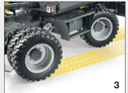
Crab steering for parallel travel along buildings.
