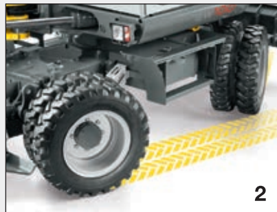
All-wheel steering for a small turning radius.
