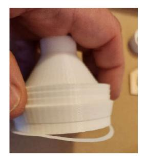
If by chance a part fits too loosely, you can apply a layer of ABS glue (see below) around the shoulder or other part and this will expand the part some to make for a tighter fit. If a part is not glued, for example the nose cone, you can also use a layer of tape to make a tighter fit.
