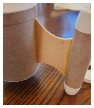
Pay attention to orientation of indentations and align in same way across 3 pods (purely for aesthetics). I recommend you install straw that connects front fins to pods as a final step since they can slide in as far as you need them to into the hole in the pods (i.e., you have some slop in their fit).
