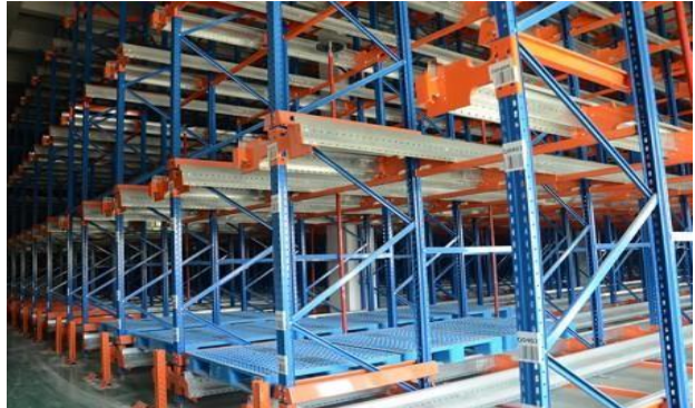
Steel radio shuttle racking for warehouse storage
