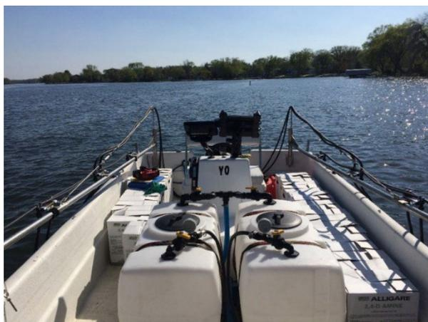
Our staff has access to five fully equipped application vessels with eight fulltime and two seasonal licensed applicators. The application will utilize our customized 18-foot Carolina Skiff boat equipped with a two-tank, sub-surface injection system. Each product tank is operated using a dedicated calibrated rate controller through an assigned set of hoses, allowing us to apply up to two different non-compatible active ingredients at the same time.
