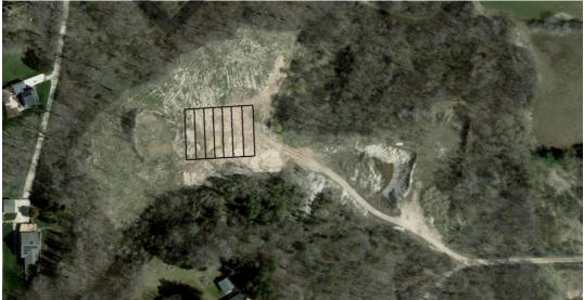
The conceptual idea utilizes 30' X 150' geotube footprint (tubes would be 60' circumference). The total necessary lay down area would then be 210' X 150' with dedicated operating space along the perimeter to support tie downs and maintenance during dewatering operations. Stacked 4 rows high utilizing 20 tubes total reaching an approximate height max of 24'. Consider the costs below:
