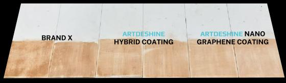
White paint with gloss clear coat Dirt Pick Up Resistant (DPUR) test according to ASTM D3719 standards.
