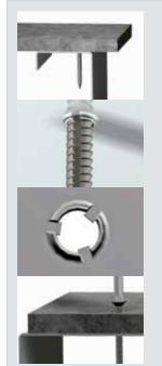
The **SCRAIL® STEELTHREAD STRUCTURAL** is driven in like a collated nail through OSB, plywood or solid wood into sheet metal with a pneumatic tool.
