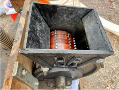
Cider making time at the mill. Slice those apples, churn them through the rotating spiked tooth scratter, press the mass of pulp and bingo: fresh, unadulterated, naturally sweet cider. Depending on the apple type, a gallon of this nectar requires about 50 apples. Much work, but a delightfully delicious pay off.
