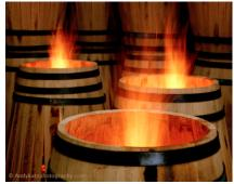
Oak barrels were used to ship whiskey as well as many other items in bulk. Making a barrel requires the wooden staves to be slowly heated so they could be bent and then fastened at the top and bottom by a metal band that pushed the staves close together, rendering the barrel watertight – or whiskey tight. Mother nature took over: these "toasted" staves imparted flavor and the reddish color to the otherwise clear distillate. How does this happen?
