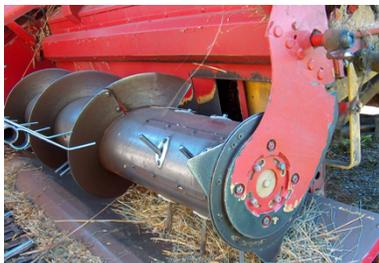
Such horizontal screws are used in farm combines to pull plants, like wheat, from the ground and feed it into a processor.
