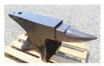
The basic blacksmith's tools have remained the same through centuries: forge, bellows, anvil, hammer, and tongs. In the forge the blacksmith heats charcoal to generate a fire; the bellows blows air to superheat and concentrate the fire. The common anvil, known as the London Pattern, has a flat face for hammering, a round front for shaping items like horseshoes, and a hole to punch holes. Hammers shape the metal, and
