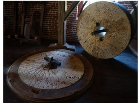
wheat berries into fine flour. While this technology has been known for many centuries, it is still an awe inspiring adventure to watch it in operation at the mill. The moving or runner stone on top must be perfectly balanced on a dime sized steel spindle protruding through the base stone. It must be perfectly balanced and level so that it maintains a paper thin separation from the base stone without ever touching it while spinning at some 80—90 revolutions per minute for hours at a time.
