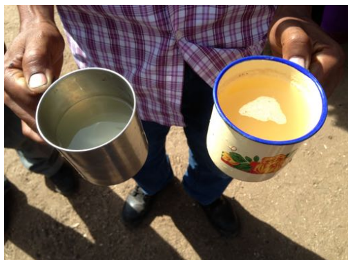
Water before and after family-size bio-sand filter
