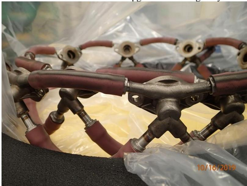
Fuel Nozzles noted fretting wear from CC Liner grommets
