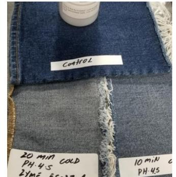
Specialty enzyme methodology can be used to lighten shades of dyed fabric. Because different enzymes can react with specific dye classes, a wide array of fashion effects becomes feasible.
