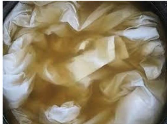
Bio-scouring is suitable as a base for dyeing of medium and dark shades, but lighter and brighter shades will need a bleach treatment to improve the base color of the fabric. This can be achieved at near neutral pH, and lower temperature by using a specially formulated enzyme and surfactant package, in combination with hydrogen peroxide.
