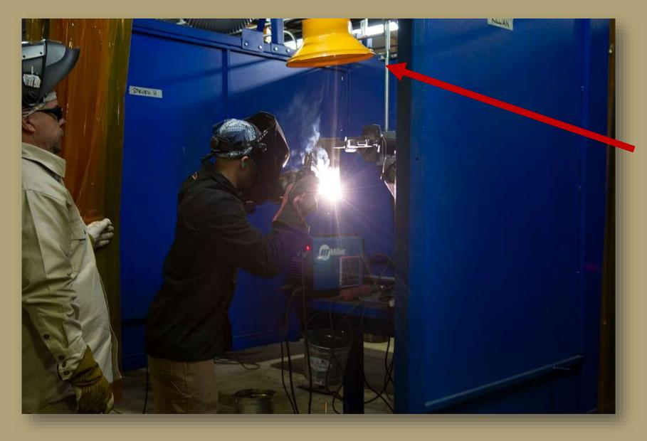
Ventilation has been installed to pull air contaminants away from the workspace.
