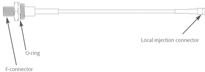
Local Injection Cable
