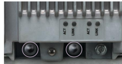
Align the RPD's alignment holes with the guide pins and seat the module
