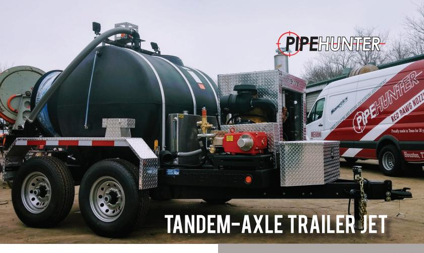
A staple in the PipeHunter Equipment line for over 25 years our first-in-class trailer jetter. This trailer jetter ranges from 500-to-700 gallons on a tandem axle trailer. The auxilary engine that drives our Giant Triplex water pump can be either gas or diesel based on the water pump specifications you choose. This engine can be equipped with 1/2", 3/4" or 1" hose with flows ranging from 18 to 60 gallons per minute.
