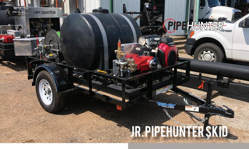
This portable skid can be put on any flatbed or in the back of a van or truck! Built to fit between the wheel wells of a pickup the PipeHunter Jr. Skid gives you jetting power on the go. This unit is built with a Giant triplex pump that will give you 3,000 PSI at 15 GPM. Our setup is great for plumbers looking to ease their way into jetting or as a hotshot rig for a municipality. To find out how this jetter can fit into your arsenal contact your local PipeHunter rep!
