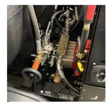
Water pump, washdown gun and hose are located on curbside between the tank and engine.
