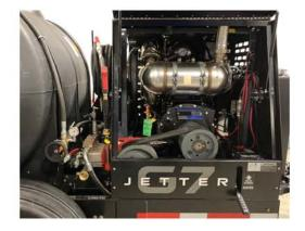
An enclosed engine compartment gives this jetter a clean look with user-friendly access for engine and water pump maintenance. A mesh screen behind the door keep the operator safe from moving parts.
