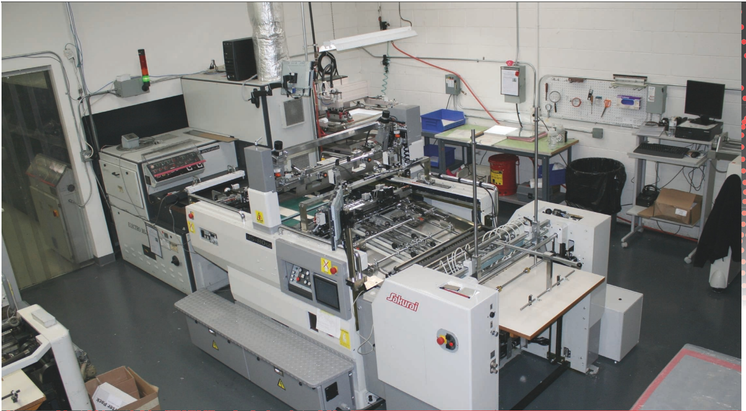
► Figure 3: This sheet-fed printing equipment can accommodate print areas from 495.3 x 635 to 495.3 x 965.2 mm (19.5 x 25–25 x 38 in). It takes sheet materials from 3 to 20 mm (0.118–0.787 in) thick. The layer-to-layer registration tolerance is 0.127–0.381 mm (0.005–0.015 in). (Source: GSI Technologies). ►
