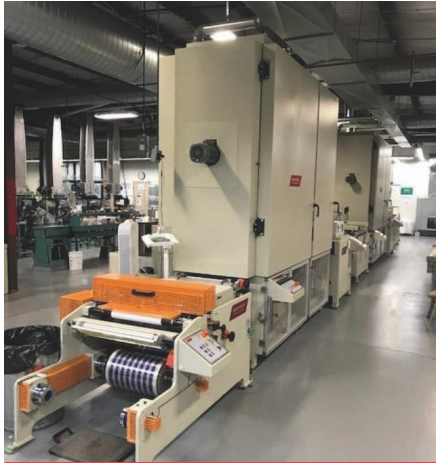
► Figure 4: This Roll-to-Roll (R2R) flatbed screen printing equipment can accommodate a print area of 495.3 x 711.2 mm (19.5 x 28 in). It takes sheet materials from 1 to 15 mm (0.039 to 0.591 in) thick. The layer-to-layer registration tolerance is 0.152 mm (0.006 in). (Source: GSI Technologies). ►
