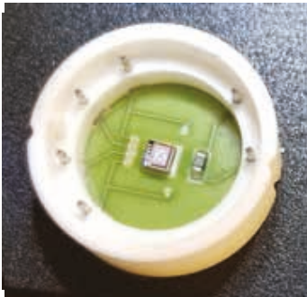
Figure 3. DunAn's TP Series sensor comprises a ceramic substrate on which a MEMS piezoresistive pressure sensor and the thermistor are mounted.
