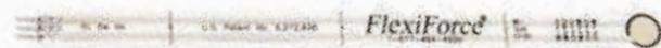
Figure 1. A high-temperature version of TEKSCAN's flexible sensor is constructed with two polyamide layers, a conductive silver layer followed by a layer of pressure-sensitive ink.
