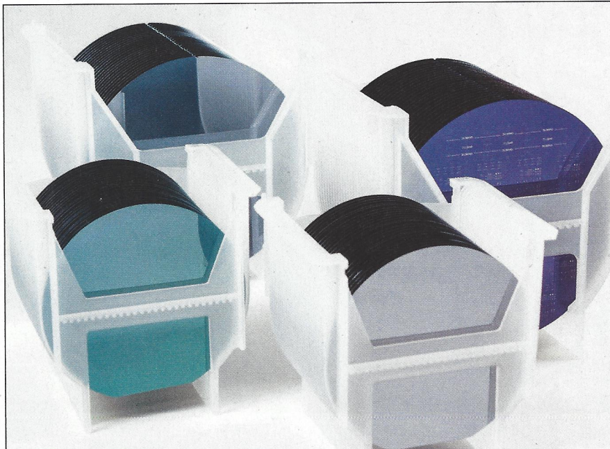
Silicon and silicon on insulator wafers are the platform from which all MEMS and semiconductor devices are manufactured. The 200mm and 300mm wafers are produced at the Okmetic's Finland facility. (Image: Okmetic)
