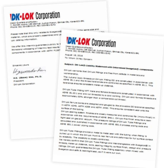
We offer this intermix guarantee publicly to the marketplace based upon TÜV Rheinland witnessing of intermix test results between DK-Lok and Swagelok® components in accordance with ASTM F1387-99(2005)
