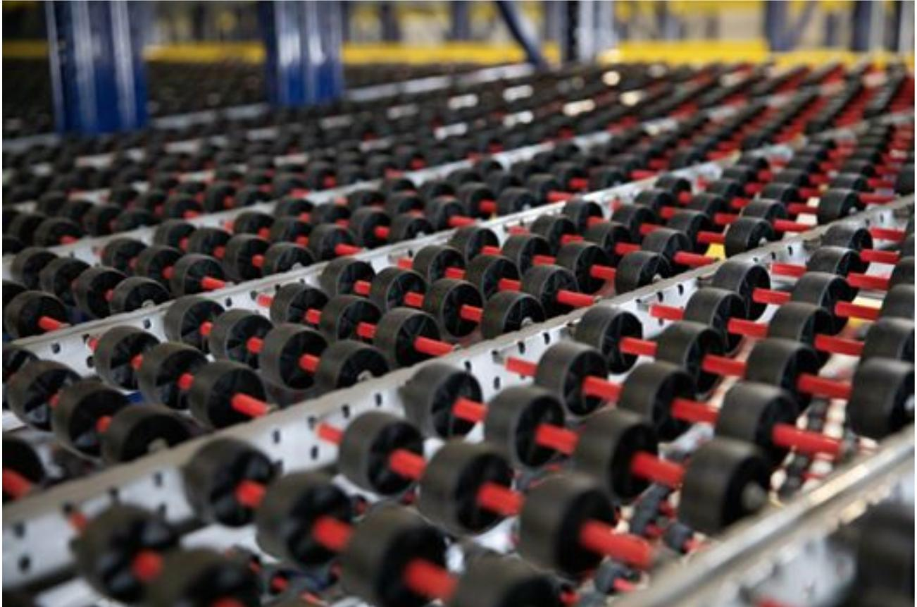
Carton flow is a form of shelving that uses a gravity that rotates products on a first in-first out inventory cycle. Product is loaded on one side and picked up on the opposite in which the next load automatically moves forward. It provides proper circulation and fast access of materials. It used for low volume case picking and for high volume split case picking.
