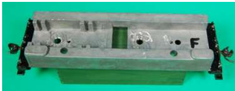
▲ The frame, with holes for the Stanton drive and decoder wires. Note the "F" to identify the front end of the frame.
