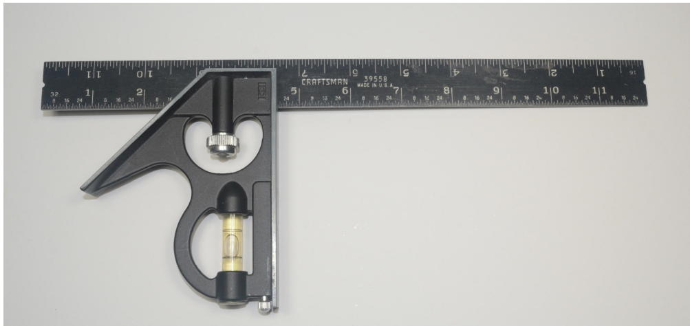
Above: My first square was a combination square. It makes square lines, general measurements and lines parallel to an edge. It helps in layout construction. I received this one recently, it belonged to my father.
