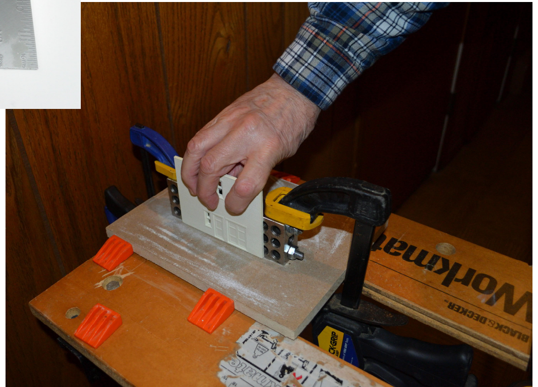
Right: Here is a sanding guide to make flat edges on walls of buildings. Using two 1-2-3 blocks makes a longer guide for the sanding operation. Holes in the blocks are used to align and join the blocks with a long bolt or threaded rod passing through the holes. The longer assembly is needed for sanding most walls.
