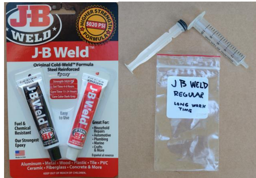
Above I like to use syringes to dispense various adhesives. I have a collection of different sizes and types and I like the controlled application. The ones with caps allow me to keep glue in the syringe and ready to use.
