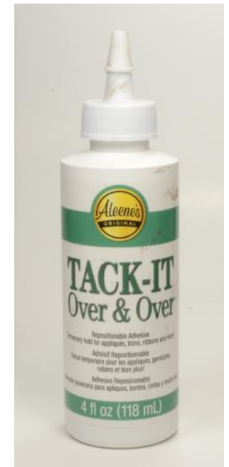
Right: Although this type of glue applies like white glue, it is allowed to dry and stays tacky. The parts are then assembled dry. Because it is so tacky be careful to keep it off unintended surfaces.
