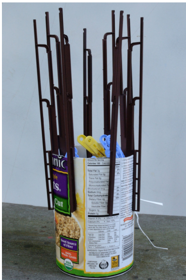
Above: A round cardboard box serves as a holding fixture for painting several parts.
