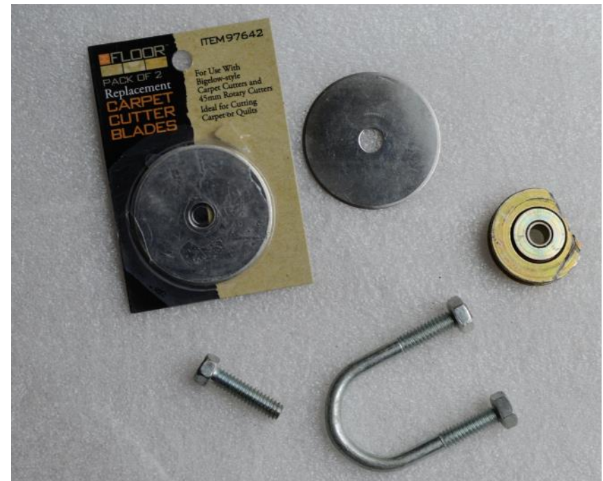
Below: The replacement blades and an assortment of parts are the elements used to make a basic rotary strip cutter.
