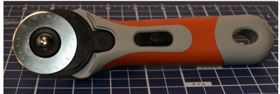
Above: This is the rotary cutter with a single blade. It is very useful for cutting aluminum foil.
