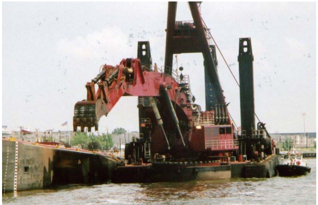
There's more than one way to dig a hole! - Great Lakes Dredge and Docks floating dredge at the Elizabeth River outlet into Arthur Kill
