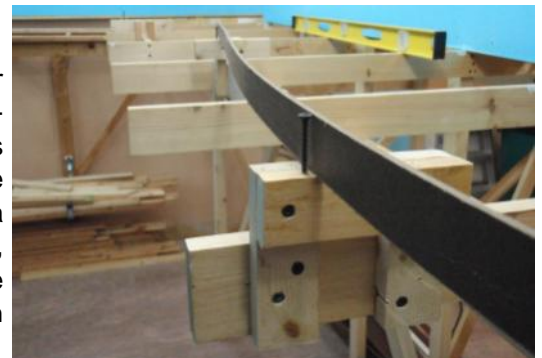
▼Screws mark the track centerline and hold a strip for the spline subroadbed in position
