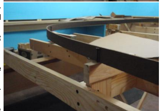
▲ A second photo showing the screws used to hold the spline subroadbed
