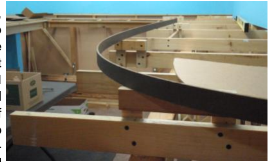
▲A strip for the spline sub roadbed shows the natural sweep of the curve
