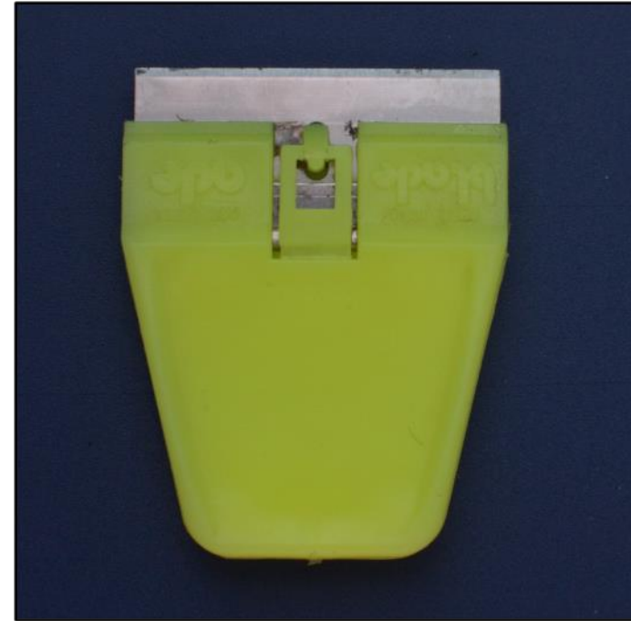
Above: Originally purchased as a scraper, this tool is a good handle for cutting with single edge razor blades.
