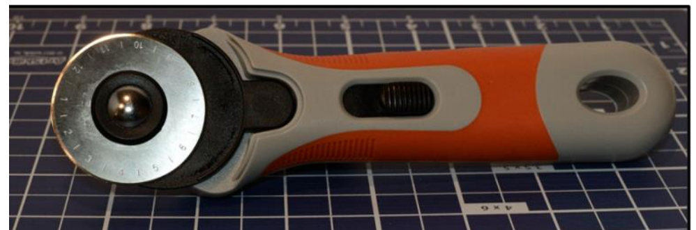
Below: Not a typical tool in a model railroader's shop, the rotary cutter is useful for cutting aluminum foil and other special materials.
