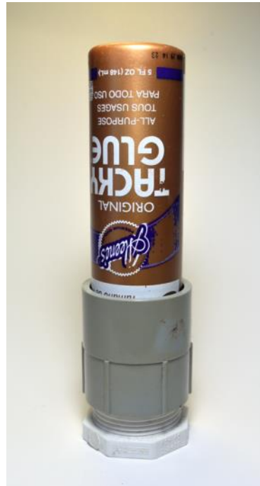
Above: A Forstner bit was used to turn some leftover PVC Window and Door Trim into the bottle holder on the left. The other two were made by repurposing corner protection packaging from a picture frame.
