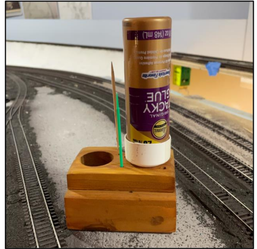
Above: Aleenes Tacky Glue is available in an inverted bottle but this stand was made to hold a regular bottle upside down. The glue is ready to use anywhere on the layout.
