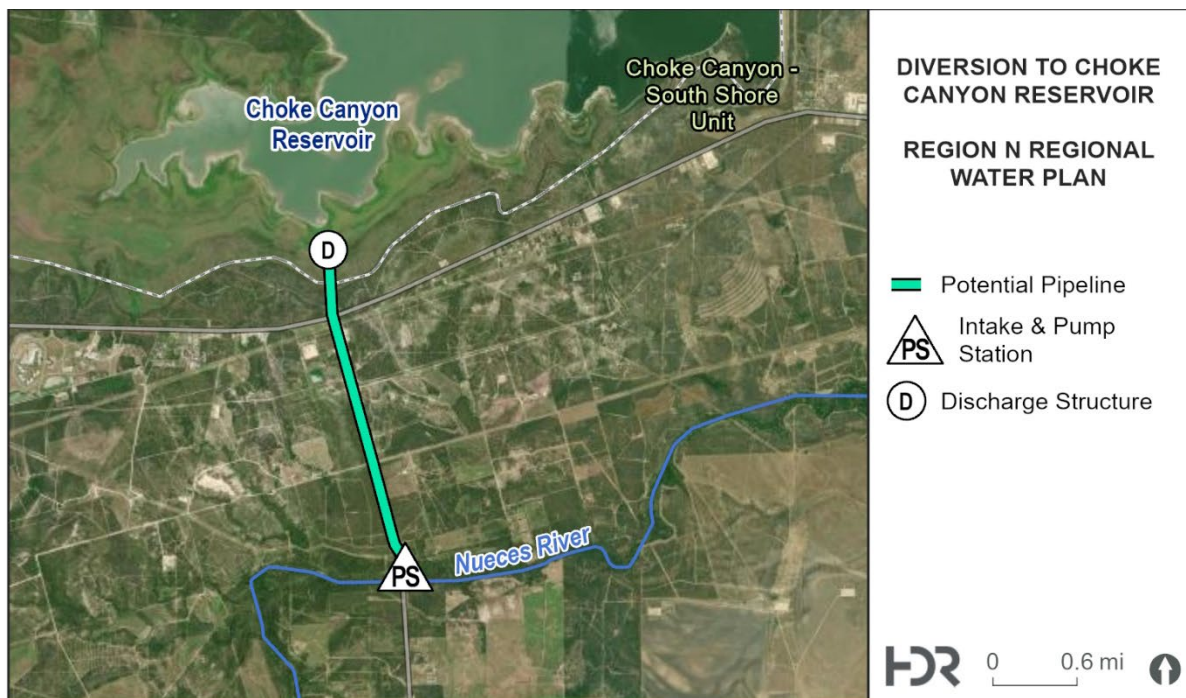
Figure 5B.11-9. Diversion to Choke Canyon Reservoir Infrastructure
