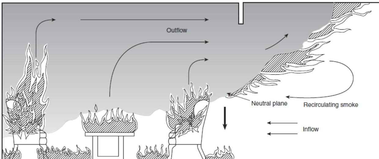
**Figure 4. Flashover conditions in a compartment fire.**
