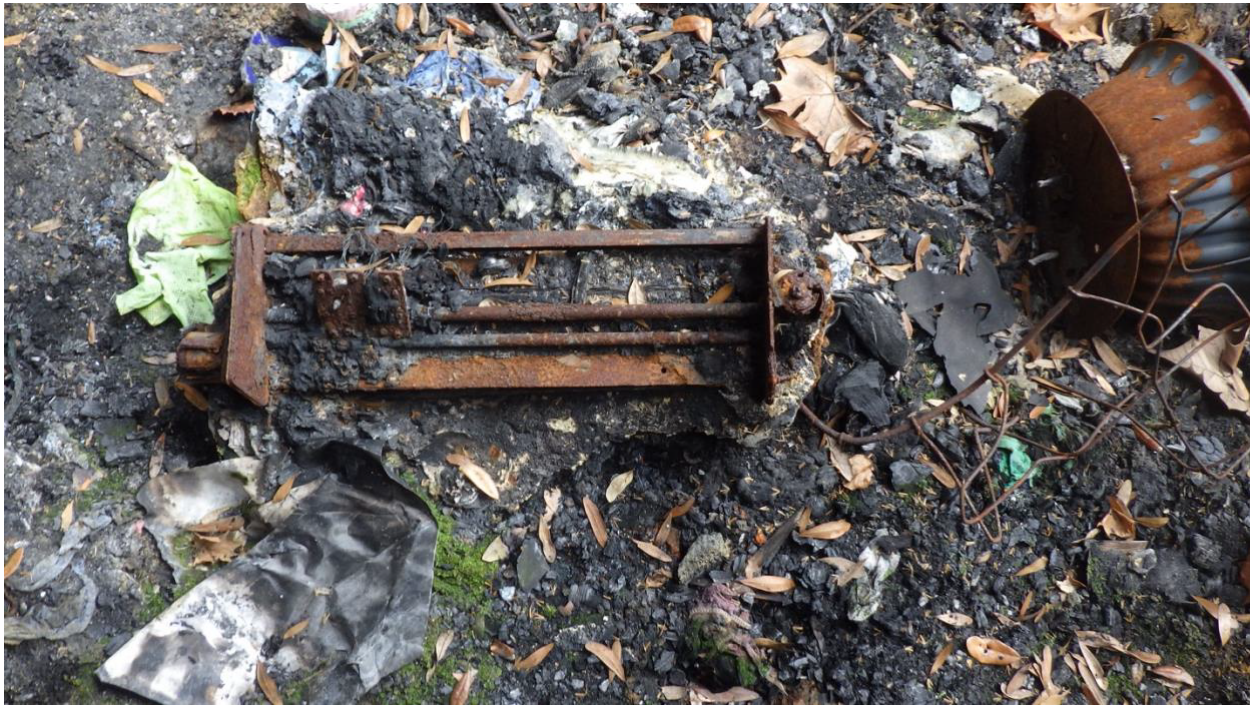
Figure 4. Mrs. [Homeowner]’s burned Cricut® machine, found during my excavation of the master bedroom. Photographed by John Lentini on February 5, 2021.
