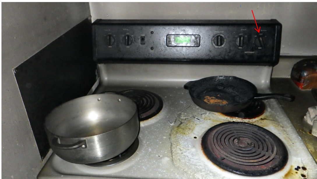
Figure 6. Closer view of the photo (JPEG) from the right side of Figure 5 , showing a halo around the right front burner, and the burner control not at 12 o'clock. Burned food is visible in the cast iron skillet, but this apparently escaped the attention of the first investigators. Overlooking critical data is one of the leading causes of incorrect origin and cause determinations.
