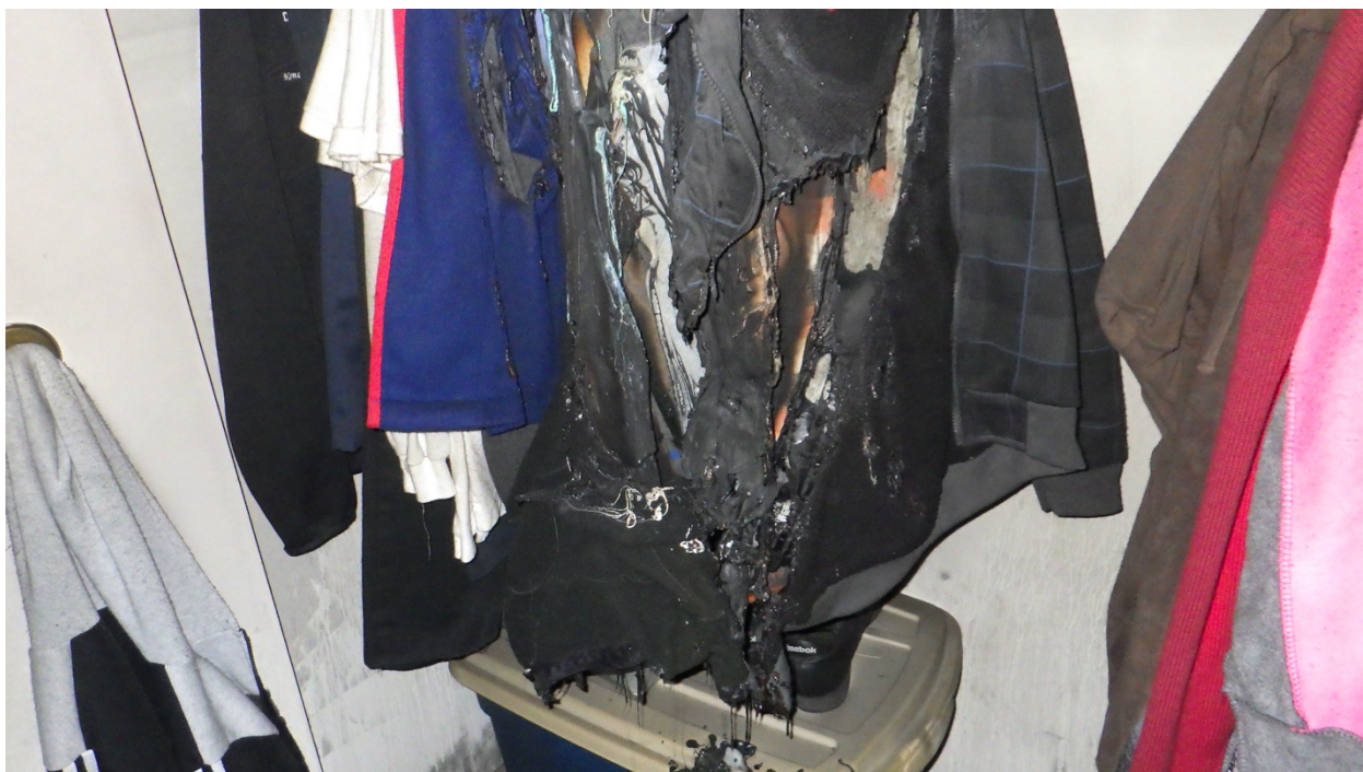
Figure 3. Isolated fire damage in the child's bedroom closet. This was identified as origin #2.
