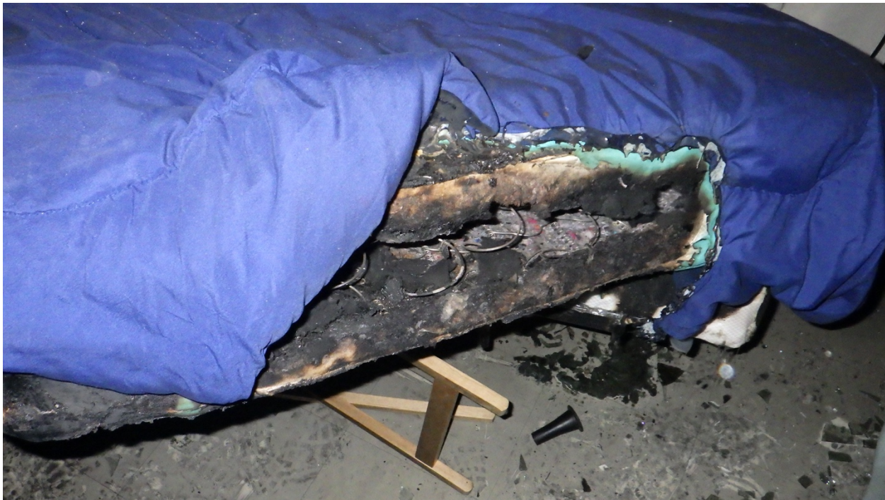
Figure 4. Isolated fire damage on the bed in the child's bedroom. This was identified as origin #3.
