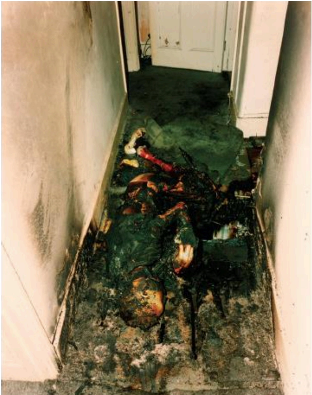
Figure 4.6 (from Scientific Protocols for Fire Investigation ) The only significant fire damage in this residence was in the immediate vicinity of the body. The victim's clothing was ignited by a small cooking fire that self-extinguished. (Photo courtesy of Mick Gardiner.)
