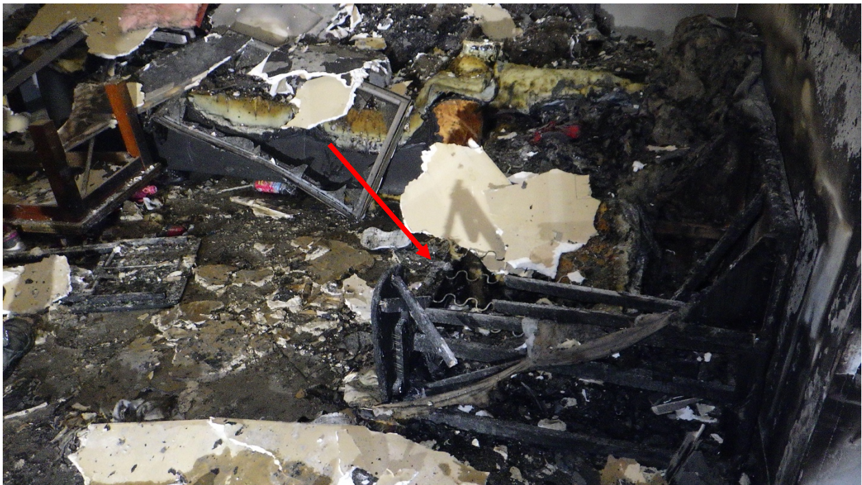
Figure 2. Fire damage on the living room L-shaped sofa. The origin was identified as being at the corner of the sofa indicated by the red arrow. The victim was found face down in front of the sofa. This was identified as origin #1.
