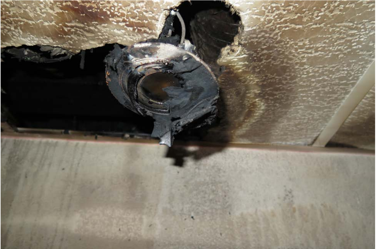
Figure 1. The cloth is clearly visible in this photo and has no innocent explanation.
