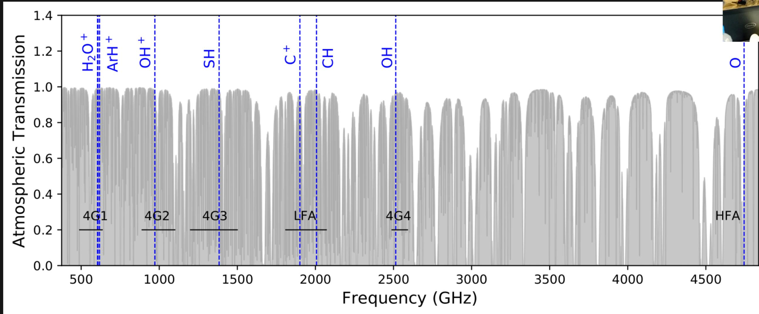
Atmospheric transmission at 38,000 feet with the HyGAL observing setups marked and labelled.
