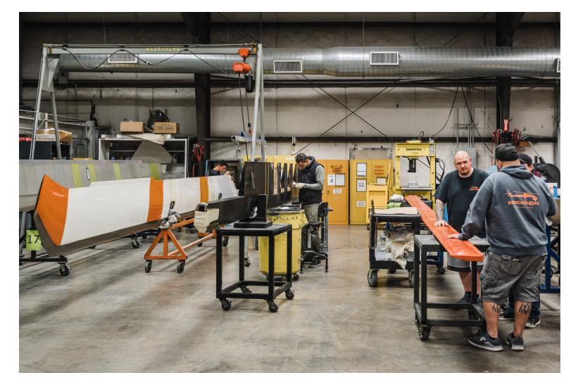
But there were other obstacles. The new blades are made with a composite material, that was provided by Toray Composites. But Johnson said that getting the layers of composite material and adhesive baked in an industrial oven at a high temperature doesn't always yield a perfect result the first time.
