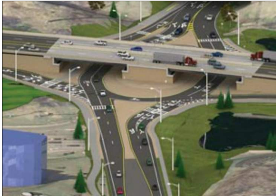
Figure B-6. Fly Over With Roundabout Underneath
