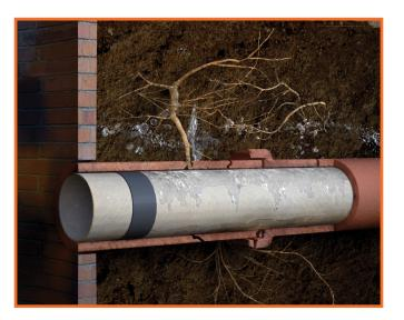
Many utilities have turned to cured-in-place pipe (CIPP) lining to address deteriorated infrastructure. Unfortunately, CIPP liners do not inherently address infiltration of groundwater, because they do not bond with the host pipe, for the following reasons:
